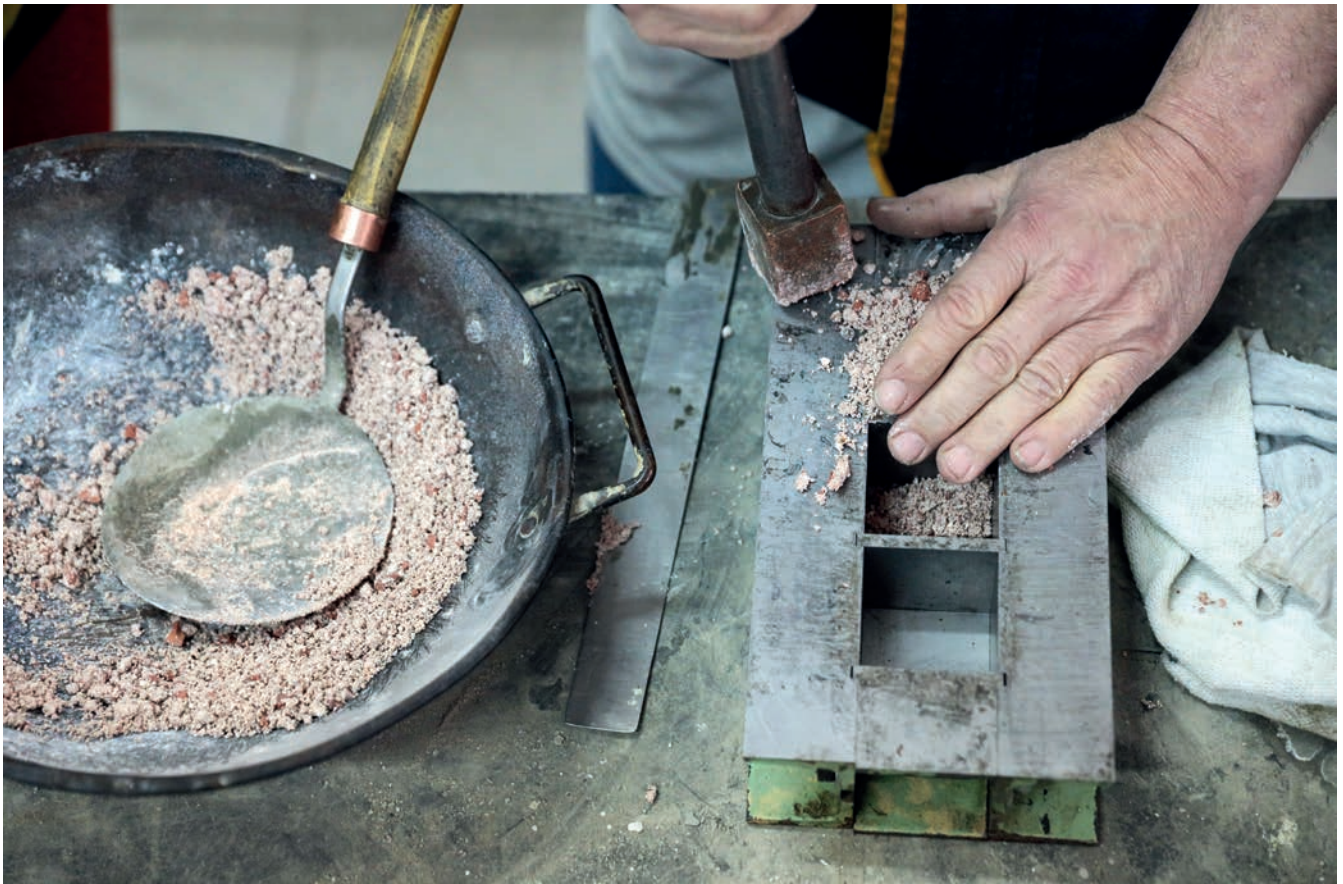
Mixing a new compatible mortar at the IMS Institute's lab
